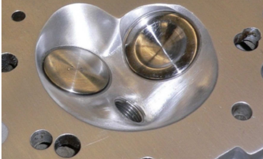
Figure 6: Combustion Chamber of High Swirl Cylinder Head
