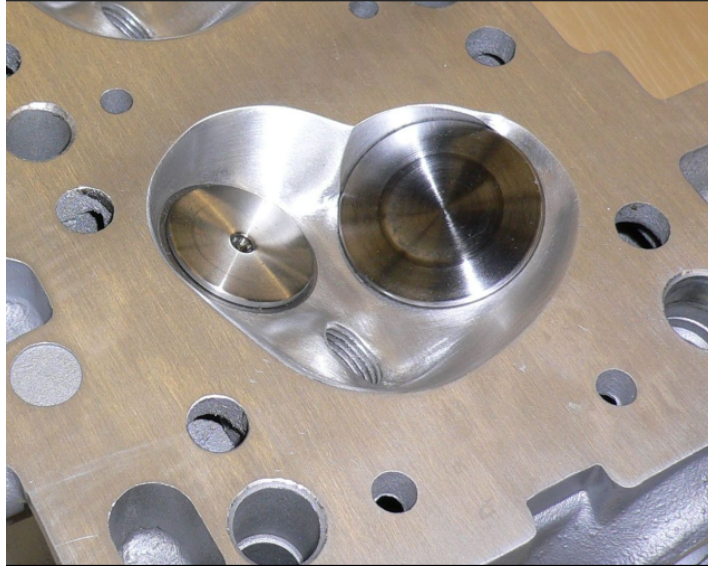
Figure 7: Combustion Chamber of Super High Swirl Cylinder Head
