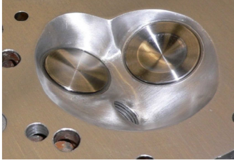
Figure 5: Combustion Chamber of Low Swirl Cylinder Head
