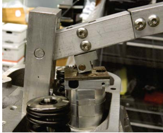
Figure 5.8. Exhaust Valve Holder and Valve Actuator Assembly on Cylinder Head.
