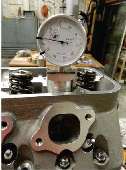
Figure 5.11. Setup using dial indicator to measure valve lift.
