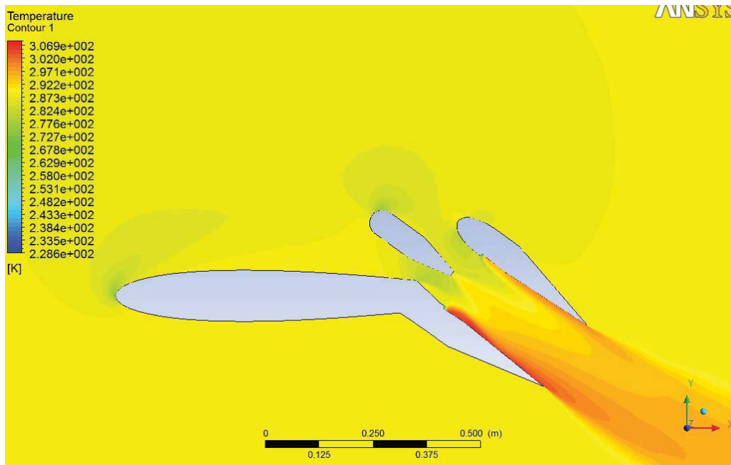
Temperature Contour: Angle 36 Mach =0.1 Wall Jets Configuration
