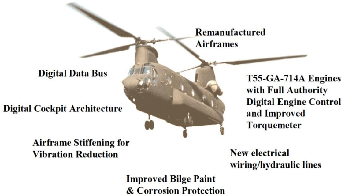
Figure 3-5. Upgraded design features of the CH-47F (Ref. 3-8)
