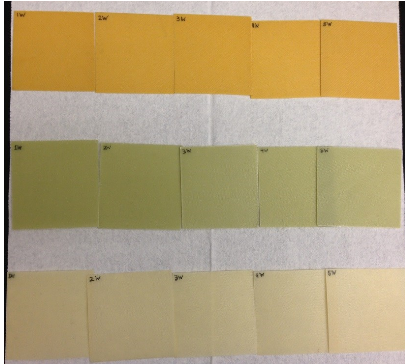
Figure 13. BMI/quartz (top), epoxy/7781 (middle), and epoxy/4180 (bottom) machined composites
