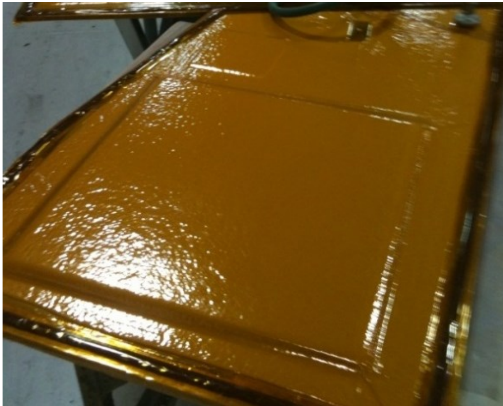
Figure 4. Actual processed BMI/quartz panel [51].
