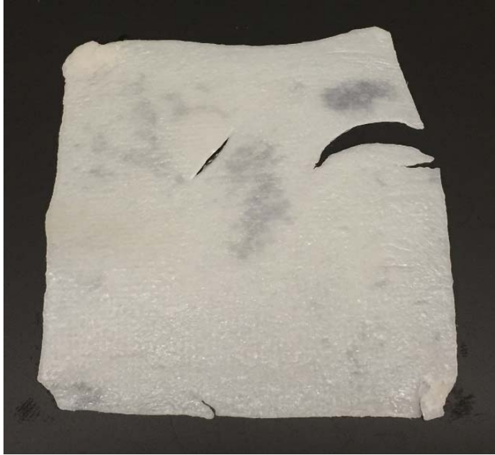
Figure 42-SIBS 72 Specimen with visible cracks due to long exposure to lipid-rich environment
