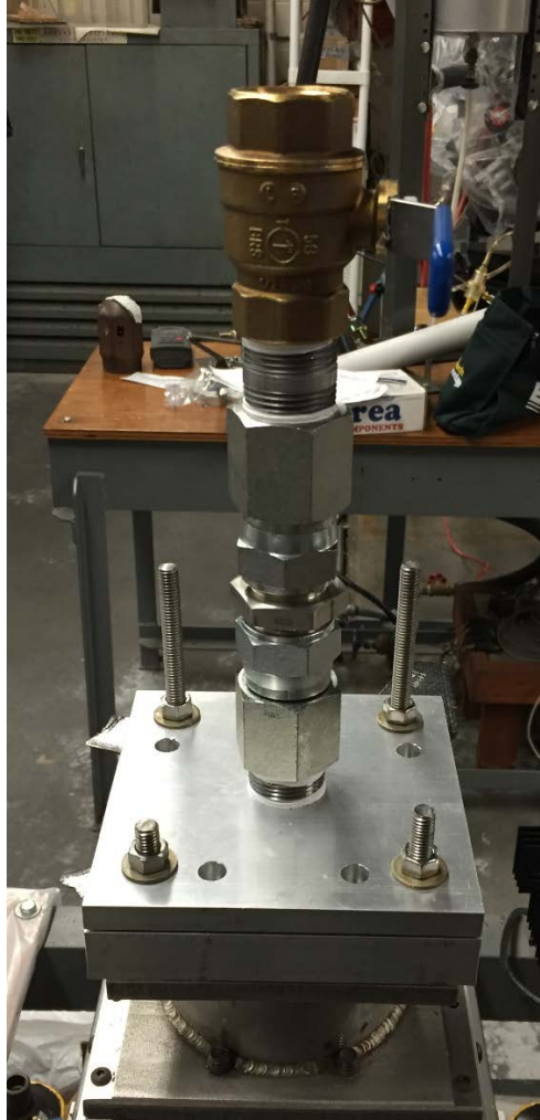
Figure 6-1 - Sonic nozzle test piece set up on the blowdown flow bench
