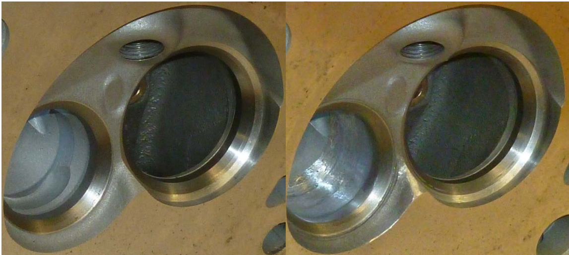
Figure 3-20 - Pictures of the stock port (left) and the modified intake side port (right)
