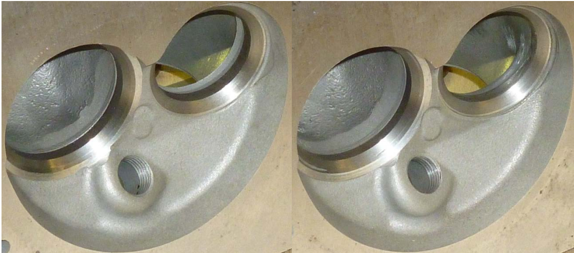
Figure 3-23 - Pictures of the stock port (left) and the modified short side port (right)
