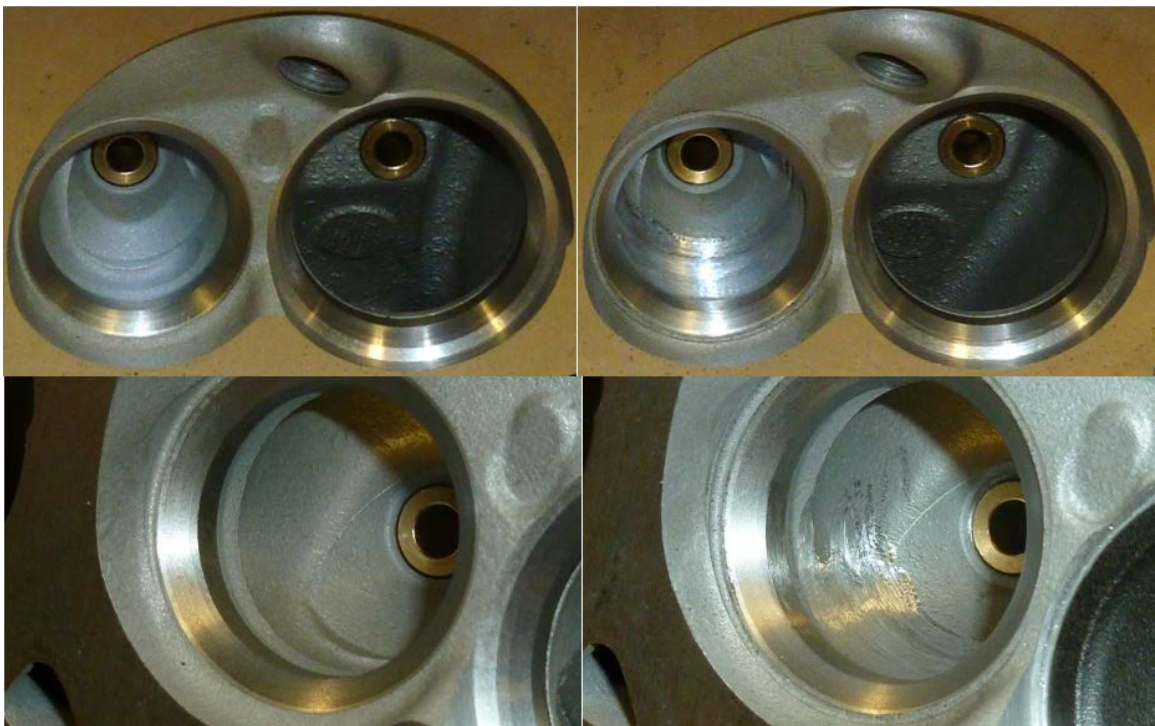
Figure 3-14 - Pictures of the stock die-cast exhaust port (left) and modified back side port (right)
