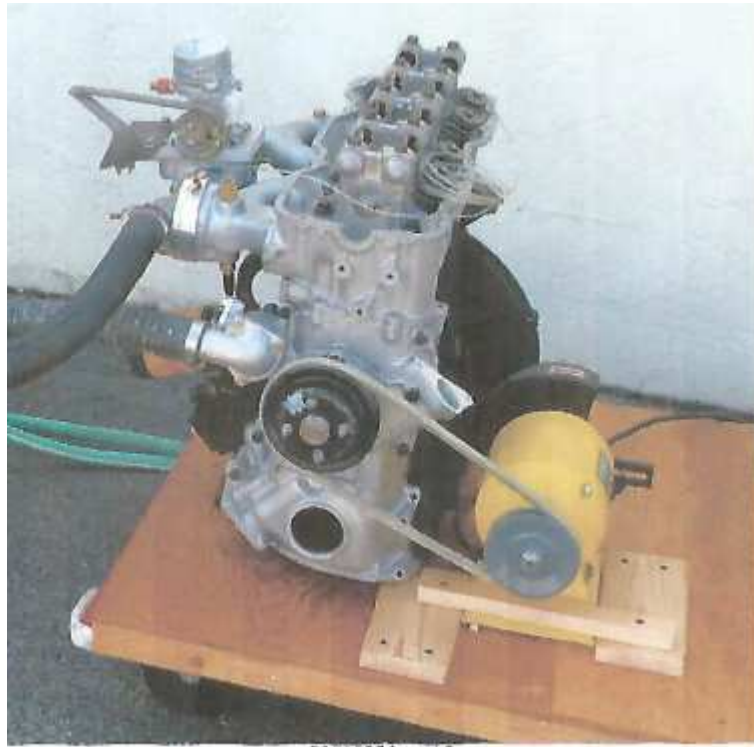
Figure 13: ASSEMBLED ENGINE FOR FLOW RATE CALCULATION
