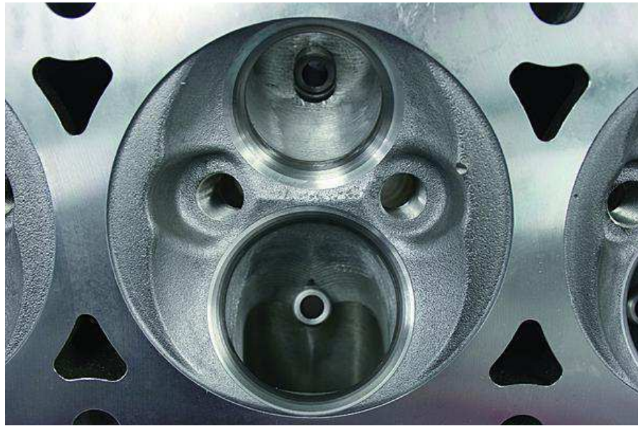
Figure 3: EXAMPLE DUAL SPARK PLUG HEAD
