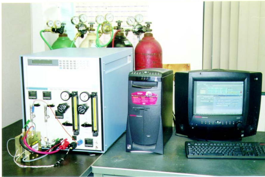
Fig. 3.1 Fuel Cell Test Station
