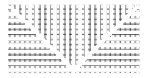
FIGURE 1 - Fishbone Racking Model Presented by Meller and Gue (2006)
