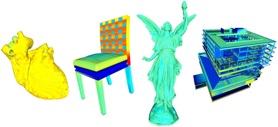
Figure 4.7: Vertices with high and low quantization levels are shown in red and blue color, respectively. From left to right: the ranges of the quantization levels are [6, 20] , [4, 21] , [12, 26] and [2, 32] bits per vertex coordinate.
