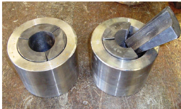
Figure 3.3: Photograph of a pair of collets with wedges.
