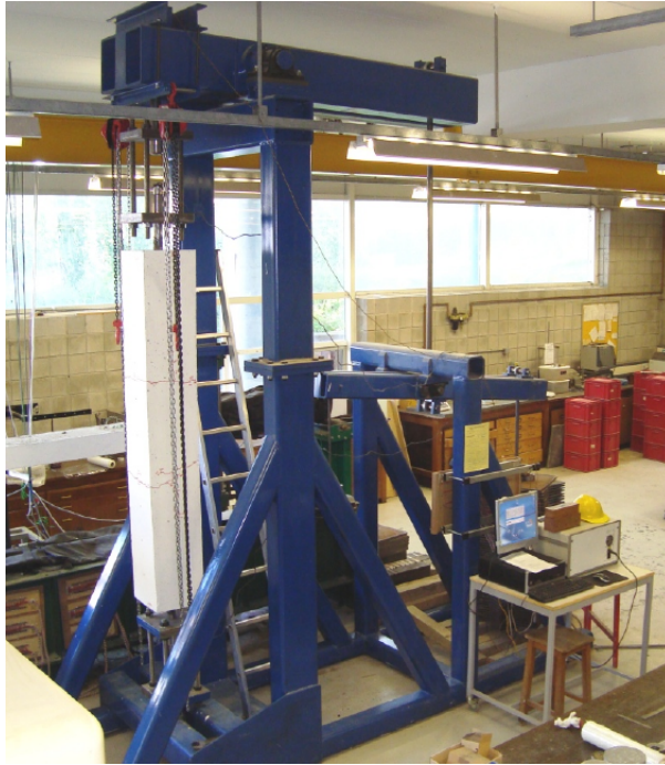
Figure 3.2: Photograph of the tension testing rig with H50 specimen under load.
