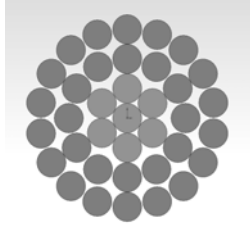
Fig. 1. The real geometry of the LYNX conductor
