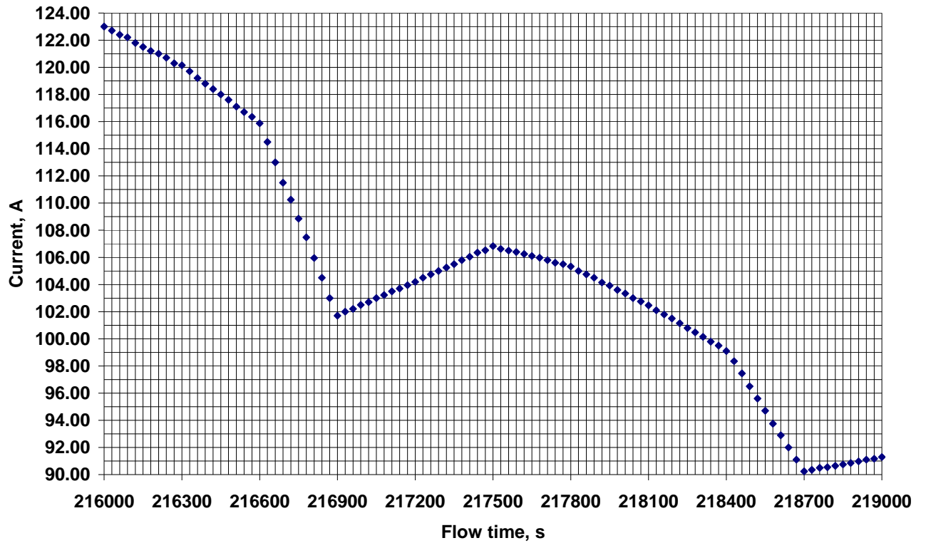
Fig. 7.15 The current variation prepared for CFD modelling
