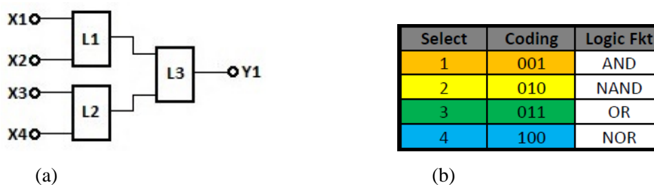
Figure 6.5: (a) Internal logic gate combination of the QLC per one clock cycle; (b) Logic function corresponding to the required selection
