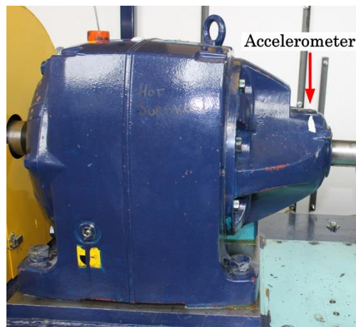
Figure 5.1: Photograph of the WTCMTR gearbox showing the location of the accelerometer on the HS end gear case.
