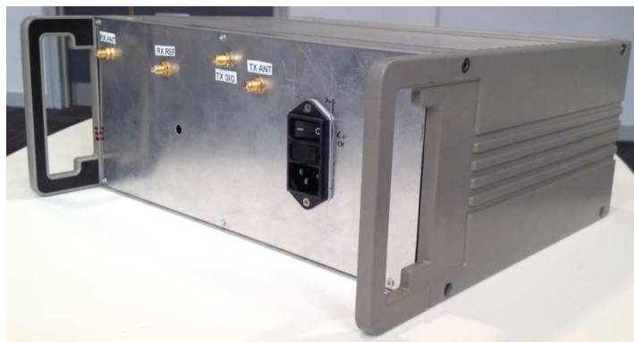
Figure 5.2: Metallic rack housing both the transmitter and receiver components.
