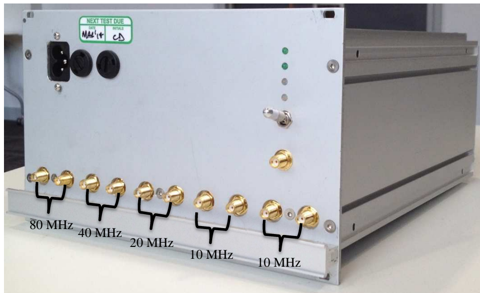
Figure 5.10: Clock distribution unit.
