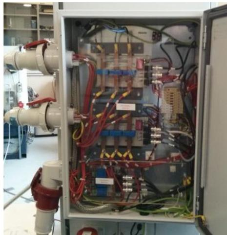
Figure 5-4 Voltage and Current Transducers
