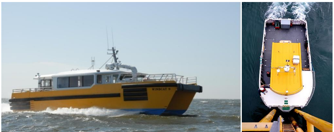
Figure 21: Examples of access by transfer boats [27].
