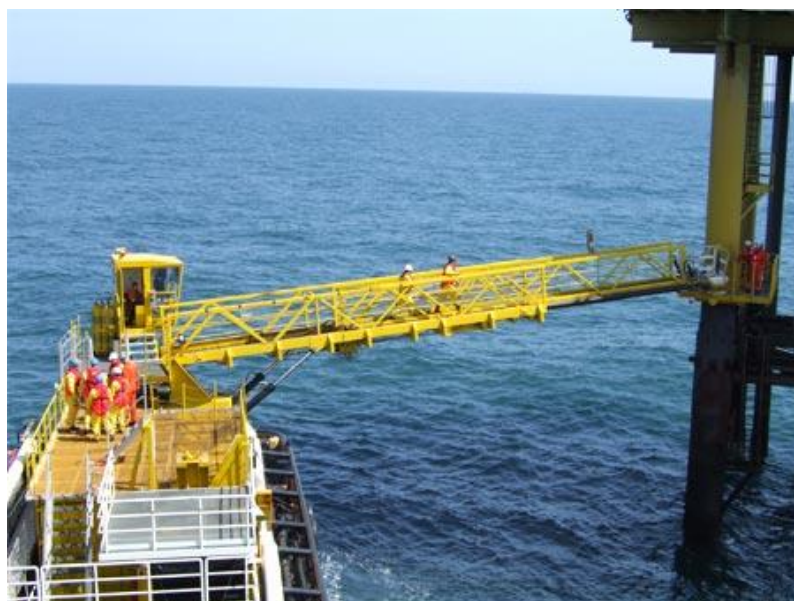
Figure 25: Offshore Access System (OAS) [30].
