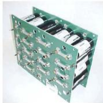
Figure 32 Ultracapacitor EPU sub module for a 1MW rated WT (Containing 32 capacitors)
