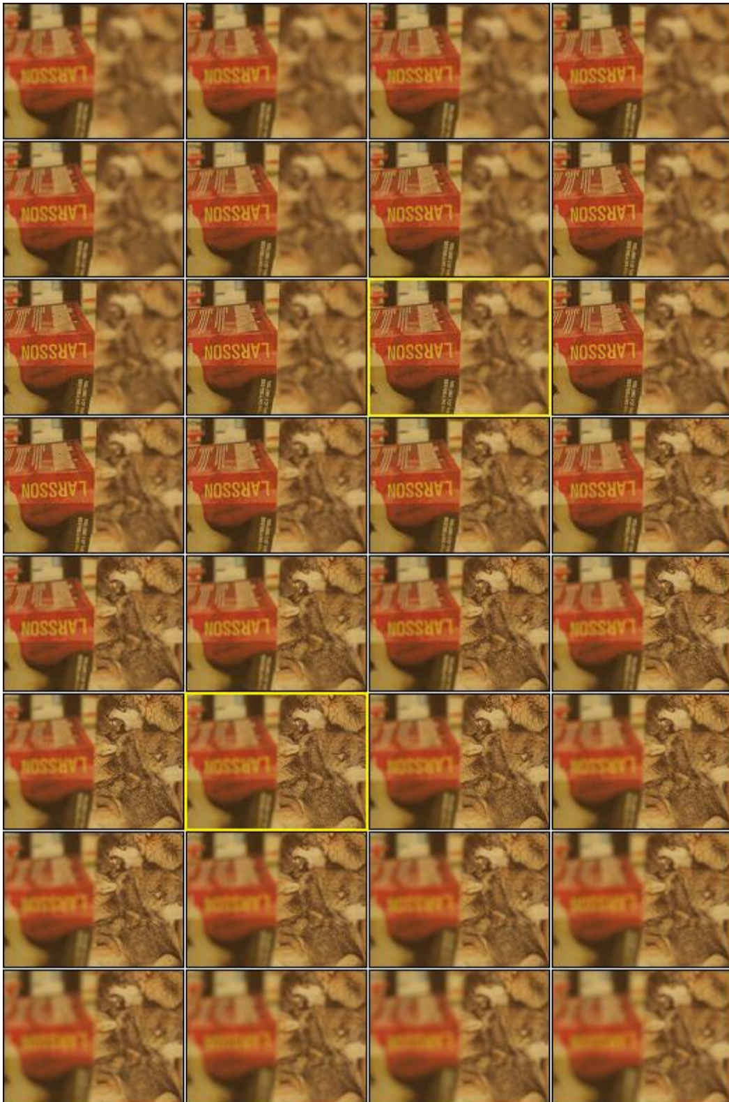
Figure 5.2.1.1.4 The 32 images in the test dataset, sequence is in rows from left to right, top to bottom. The first plane comes into best focus in image 11 (highlighted in yellow) and the second plane comes into best focus in image 22 (also highlighted in yellow).
