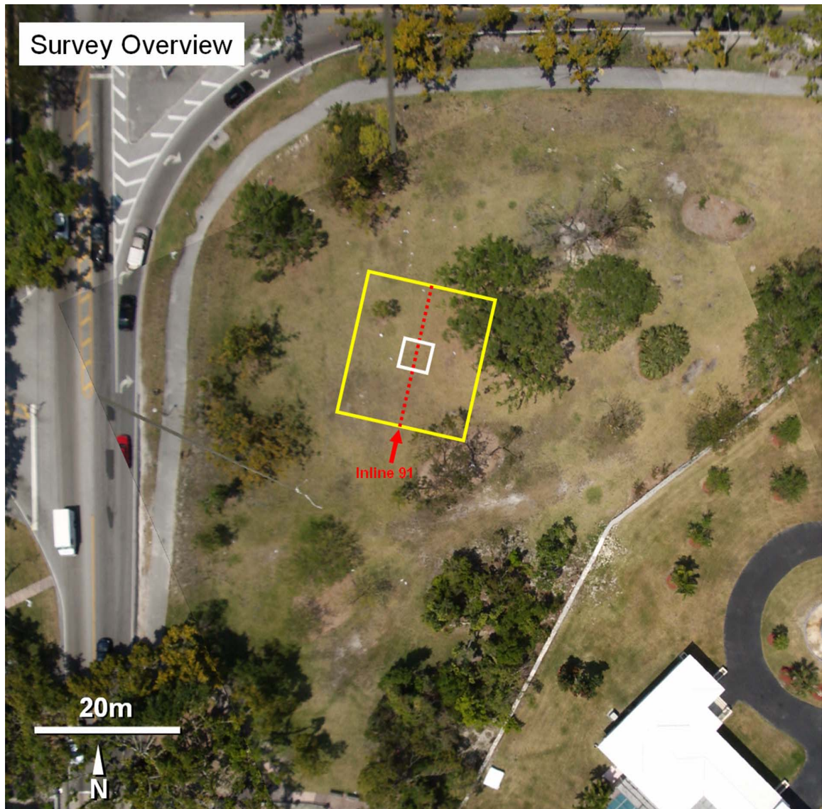
Figure 5.1: Aerial photo of Ingraham Park in Coral Gables, FL with overview of 4D GPR experiment. The large box outlines the 18 x 20 m survey area, while the small box outlines the 4 x 4 m pond area where 3200 L of water were injected. The dotted line indicates the location of an extracted line of the GPR data.
