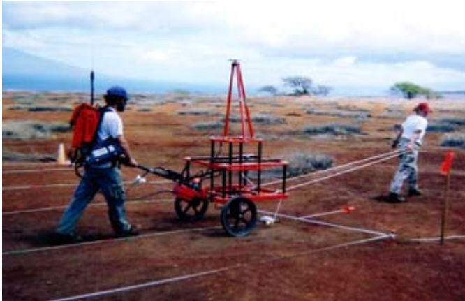
Figure 2.1: Photo showing typical GPR data acquisition with the assistance of measuring tapes staked out on the ground to guide the user along target transects [11]. Such acquisition is tedious and compromises are often made to save time by recording less data and interpolating.
