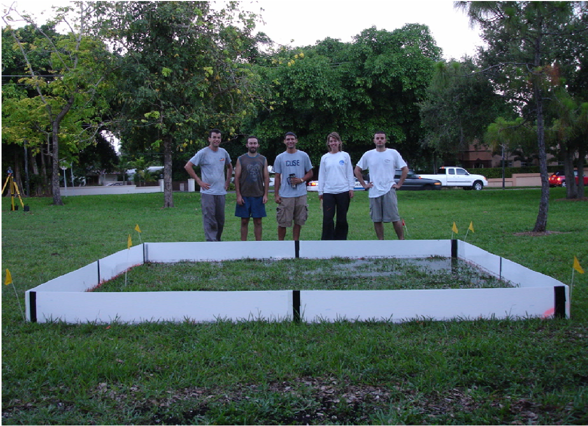
Figure 5.2: Photo of the 4 x 4 m artificial pond and the five participants of the 4D GPR experiment. 3200 L of water were injected into the pond over a period of 4 hours so the infiltration of the water into the shallow subsurface could be tracked using repeated 3D GPR surveys.
