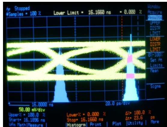
Fig. 5.12. The full width of the time histogram for p-p jitter.
