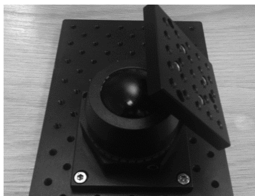
Fig. 3.3. The sample/mask plate holder with rotation features for multi-directional inclined UV exposure.
