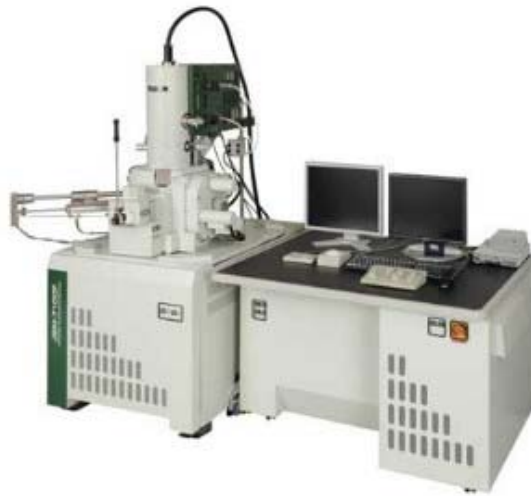
Figure 5.3 JSM-7100F Scanning Electron Microscope.
