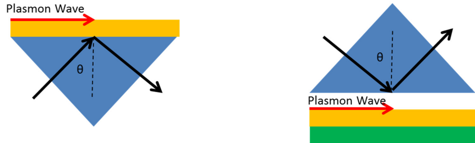
Figure 2.5 surface plasmon excitation through prism coupling in the Kretschmann (left) and Otto (right) configuration.
