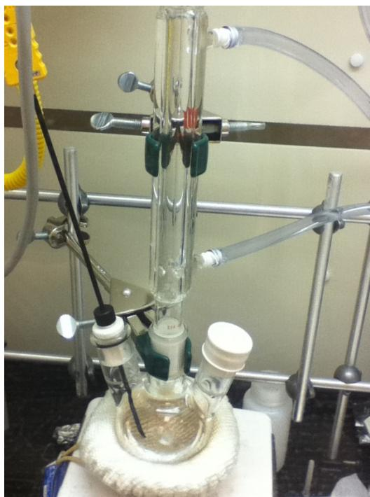
**Figure 3. 5** QD synthetic apparatus employed in the preparation of CQDs by the hot-injection method.
