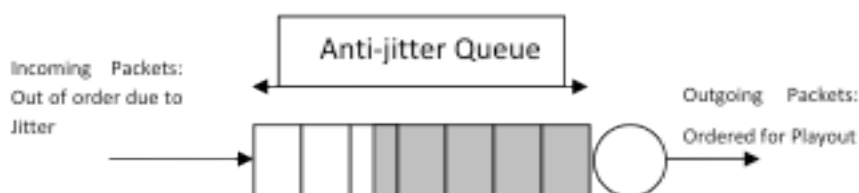
Figure 1.4: Mechanics of the Anti-Jitter Buffer
