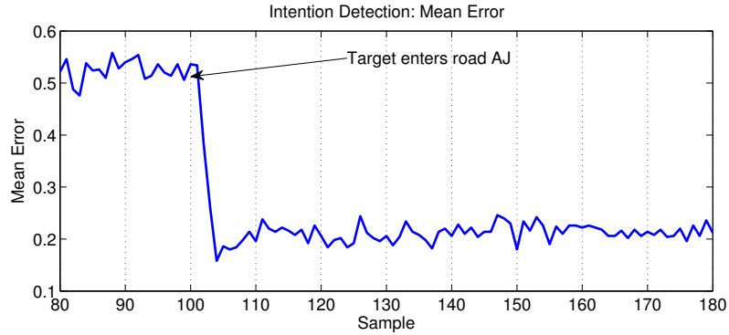
Figure 5.8: Probability of error (MSE) in intention detection when the DS-based model is used (500 trials). The mean error is a function of the uncertainty intervals in Table 5.3.
