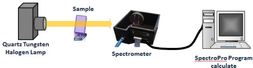
Figure 3.7 The absorption spectra measurement using a spectrometer and a halogen lamp.
