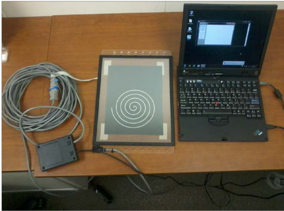
Figure 3-2: Spiral recording setup.
