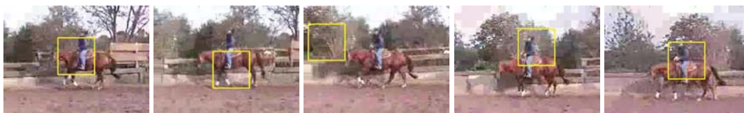
Figure 5.4: Moving object detection in a sampled video sequence (frame sampling rate is 3 fps)
