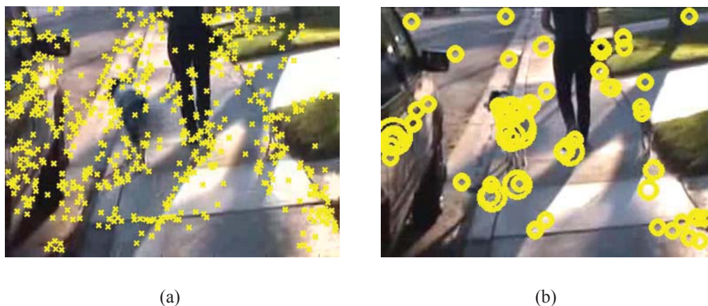
Figure 4.31: Comparison of interest point distribution. (a) interest points detected by difference of Gaussians edge detector are illustrated in yellow crosses; (b) interest points detected by Harris3D detector are illustrated in yellow circles.
