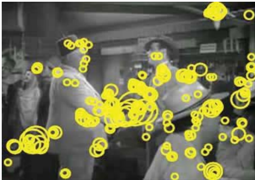
Figure 2.3: Space-time interest points detected for a video clip with human action - hand shake [3].
