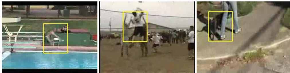
(b) Region of motion detected by local motion estimation layer based on 4.33(a)
