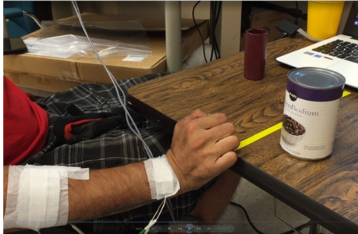
Figure 6.2 Subject readying to perform the Grasp and Release Test. Stimulation is delivered to the muscles responsible for opening and closing of the hand, so that the subject may grasp the object, pick it up, and move it from one side of the table to the other.
