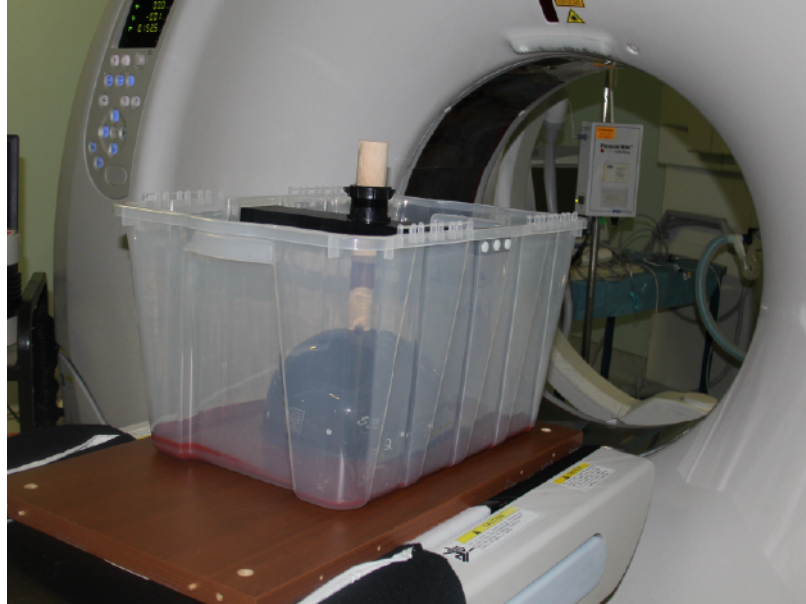
Figure 14: Helmet positioned in fixture with poured silicone rubber as the base and a wooden dowel to maintain the helmet's position. No saline solution has been added here.
