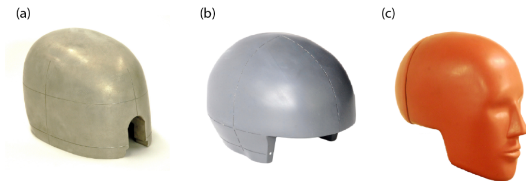
Figure 2: Examples of common head forms. (a) The metallic headform defined by the US Department of Transportation standard (DOT headform); (b) The metallic headform defined International Organization for Standardization (ISO headform); (c) The vinyl-covered metallic headform used for the Hybrid III anthropomorphic test device or crash test dummy. The latter headform is commonly used during automotive crash testing.
