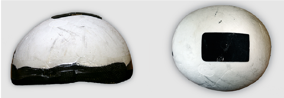
Figure 19: Foam liner from 2XL helmet containing additional foam segment at vertex.
