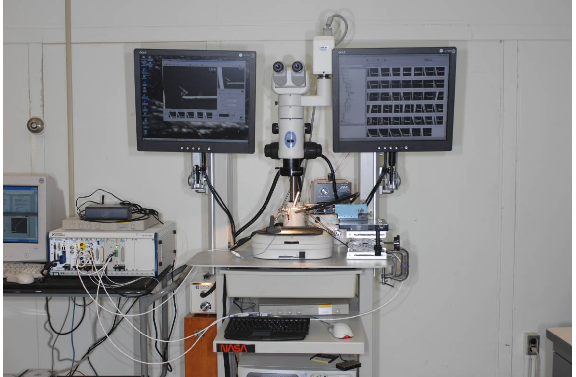
Figure 4-1 Tin whisker test station - full experiment
