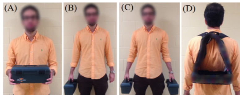
Figure 13. Carrying methods investigated: (A) Frontal, (B) Lateral, (C) Bilateral, and (D) Posterior. Note that a hole was made in the backpack to allow the motion capturing system to capture the T10 reflective marker.
