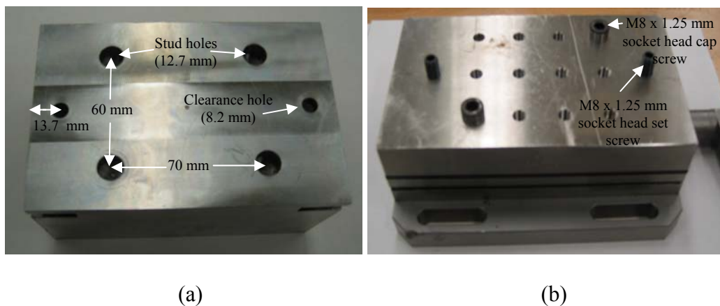
Figure 3-17 (a) Clearance and blind holes drilled in the bottom of the block, and (b) Socket head set screws and cap screw on dynamometer plate
