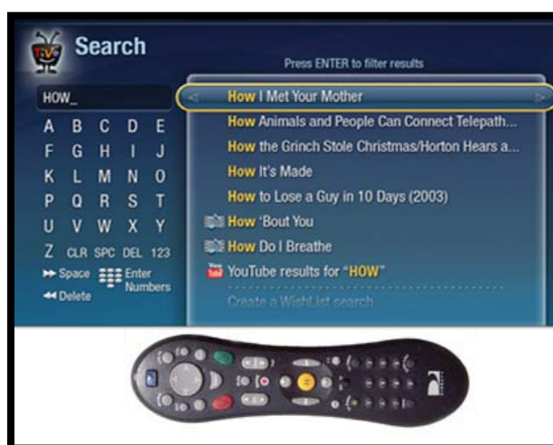
Figure 2-8 Tivo DVR Uses Five Keys and an On-screen Keyboard for Text Entry
