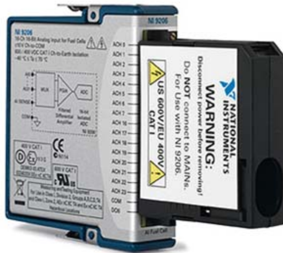
Figure 3-23 National Instruments 9206 16 channel analog voltage input module.
