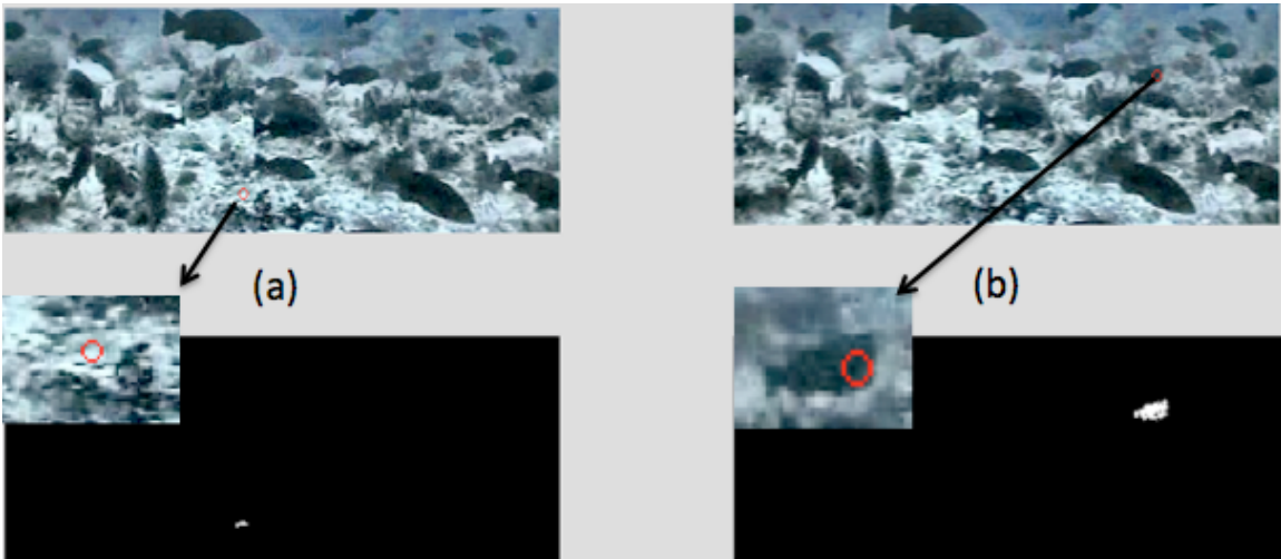
Figure 4.16: Region growing on seafloor (a) and fish (b).
