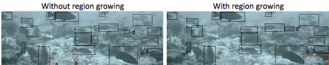
Figure 4.17: Detection and region growing to resolve broken fish regions
