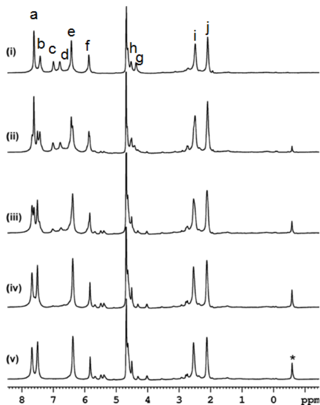
Figure 4.1 ^1\text{H} NMR titration experiments of 2-methoxynaphthalene ( 1a ) with host OA. (i) OA (1 mM in 10 mM buffered \text{D}_2\text{O} ), OA/2-methoxynaphthalene at (ii) 4:1, (iii) 4:2, (iv) 4:3, and (v) 4:4. Aliphatic guest resonances are marked with *.
