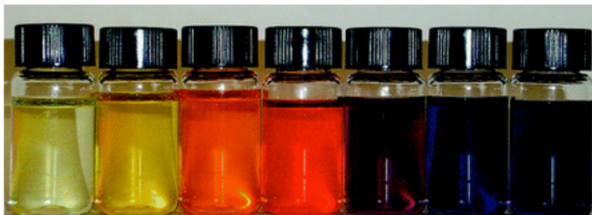
Figure 1.1 Colors of the \text{Mo}(\text{P}^i\text{Pr}_3)_2(\text{CO})_3(\text{RCN}) complexes studied. From left to right: R = Ad; 4-NMe 2 C 6 H 4 ; 2,4,6-Me 3 C 6 H 2 ; C 6 H 5 ; 2,6-F 2 C 6 H 3 ; 4-CF 3 C 6 H 4 ; F 5 C 6 .
