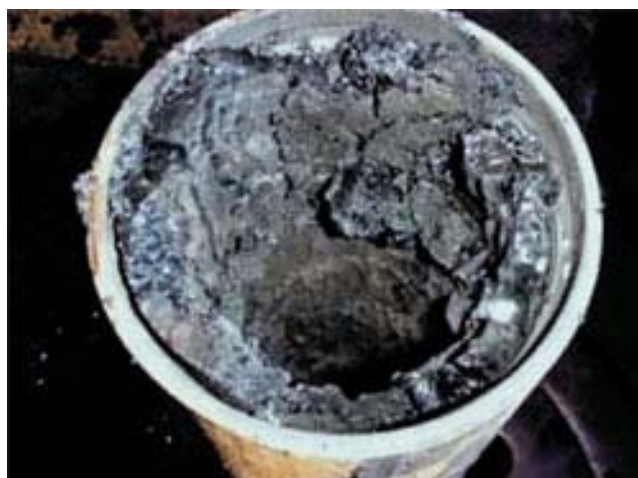
Figure 4.2. Main crude oil component, asphaltene, leading to pipe obstruction.
