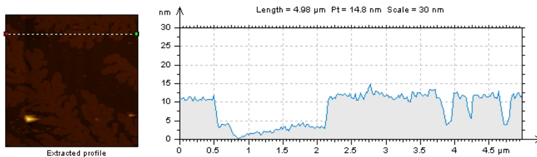
Figure 3.3 Profile extraction analysis of Pluronic F-127 deposited on mica.
