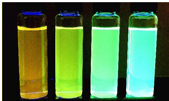
Figure 3.11 Orange CDs aqueous dispersion under the irradiation of UV light (365 nm). From left to right, orange CDs were dispersed in water, methanol, acetone and THF.
