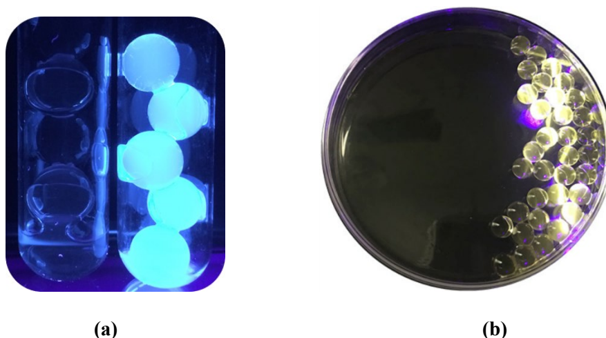
Figure 6.2 Orbeez beads treated by (a) water (left), gel-like CDs aqueous dispersion (0.1 mg/mL) (right), and (b) orange CDs aqueous dispersion (0.1 mg/mL) irradiated by UV light (365).
