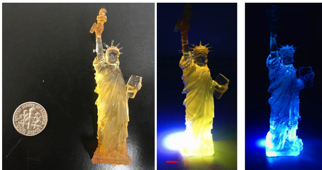
Figure 6.3 (a) The comparison of the printed figure with a one-dime coin; (b) 3D printing of “statue of liberty” with CDs-SAP conjugate (left) and control without orange CDs (right).
