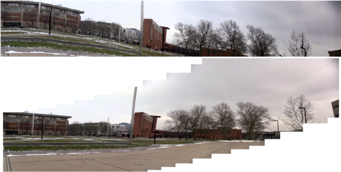
Figure 7.1.: The profile (top) and spatial mosaic (bottom) of videos with continuous camera operation (pan right with tilt up) with camera pan as major operation. The continuous up-tilt operation can be seen from the profile (top) as the decline of the structure line toward right. The spatial mosaic (bottom) cannot fit in the time line of video editing software due to the irregular shape caused by various camera operations.
