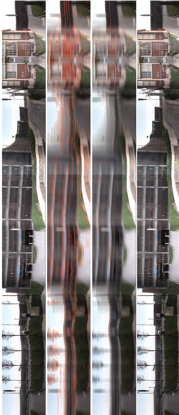
Figure 7.8.: The process to rectify video profile with distance feature long lasting in the shape-oriented condensed image C_x(t, y) . Video profile, C_x with tracked traces (red), the longest traces (red) in C_x , and video profile after straightening according to the longest traces are displayed from left to right. The method works for wide area.
