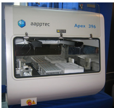
Figure 1.10. AAPTEC Apex 396 fully automated peptide synthesizer.
