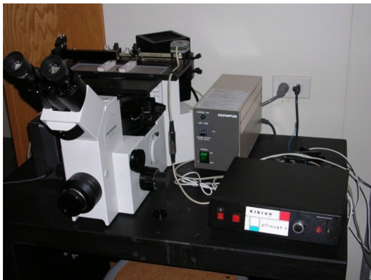
Figure 1.4. Olympus IX-70 inverted microscope with Kibron trough for the acquisition of epifluorescence microscopic images.
