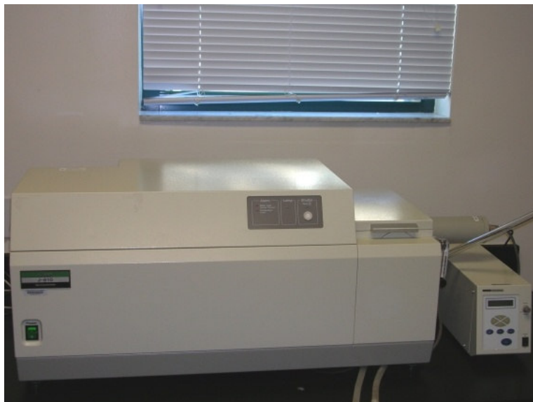
Figure 1.8. Jasco J-810 circular dichroism spectrometer.
