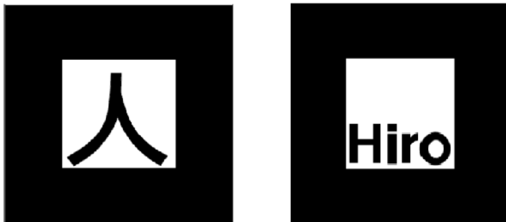
Figure 3.2 Commonly used patterns in vision-based tracking – kanji pattern and hiro pattern [44]
