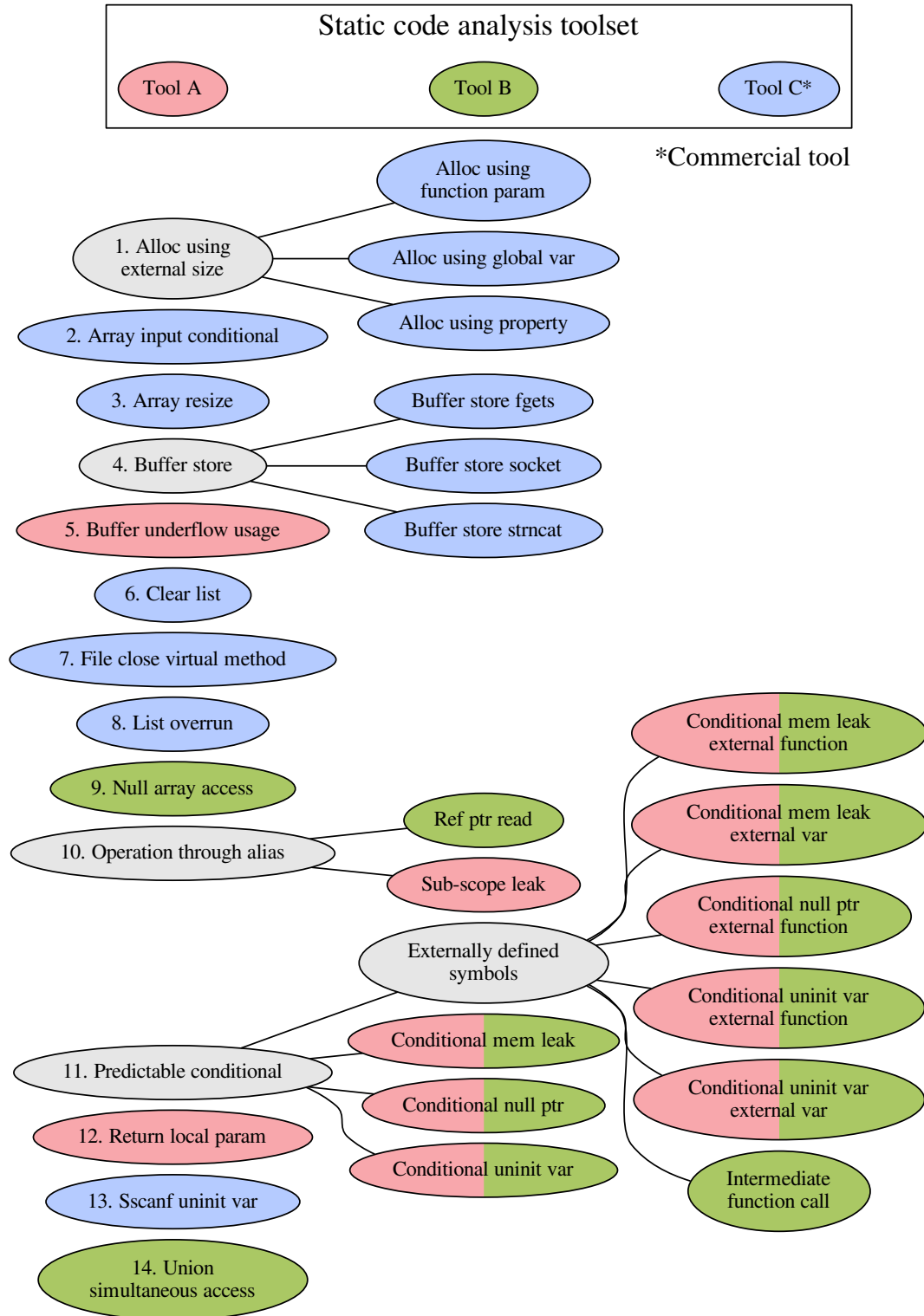
Figure 4.1.: Hierarchy of identified false positive patterns when executing static code analysis tools against the Juliet test suite. The 14 core false positive patterns or pattern families are numbered in the first column.
