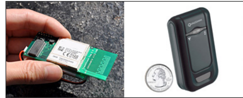
Figure 7: Trash Track Tags (left) that use cellular Technology to report location of discarded Item. Courtesy of SENSEable City Lab.
