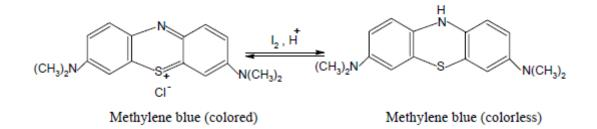
Figure 1: The de-colorization reaction of Methylene blue
