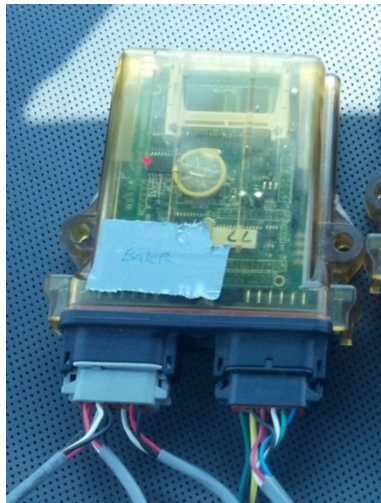
Figure 3.8 CyCAN Data Logger Used to Capture TG 305 Tractor and Baler Data During Double Pass Harvesting
