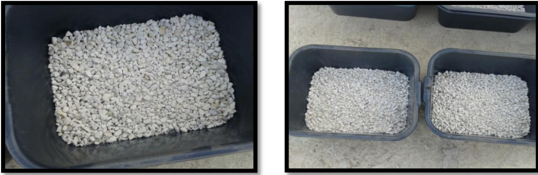
Figure (3.7): Filling container with the first layer of large gravels.
